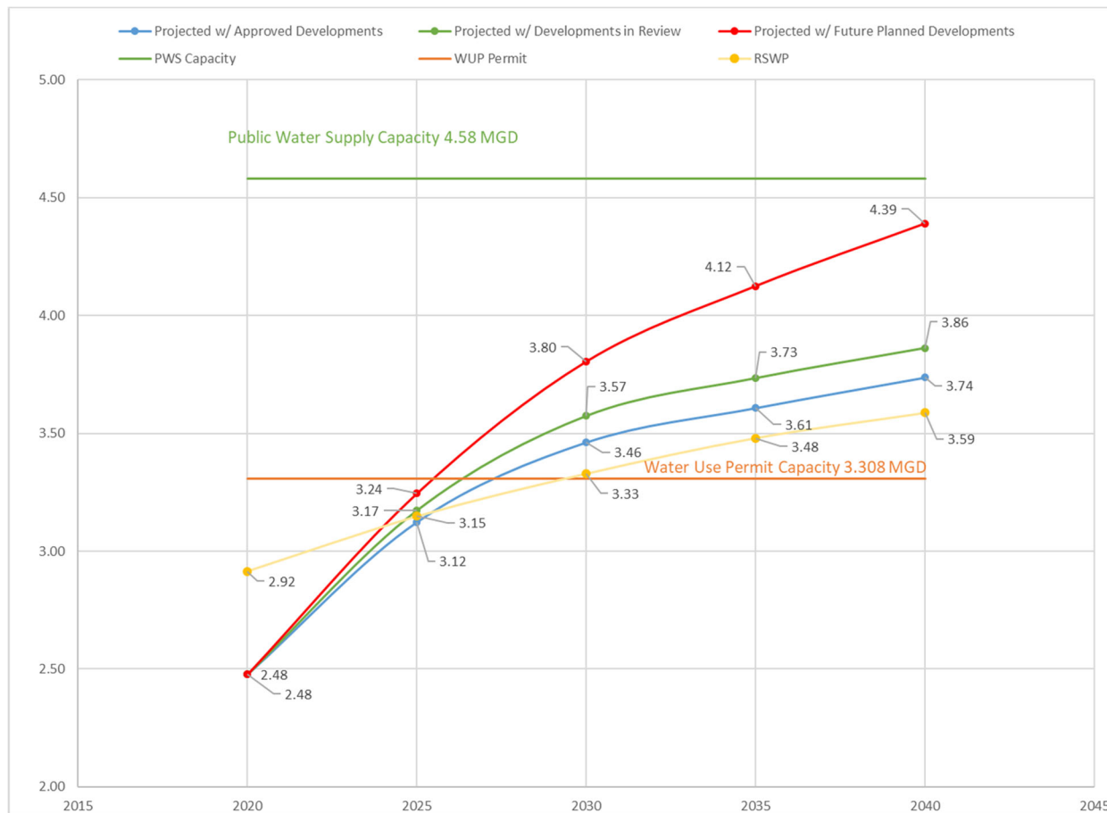
Figure 2 Projected Potable Water Demands and Capacities, City of Zephyrhills USA
