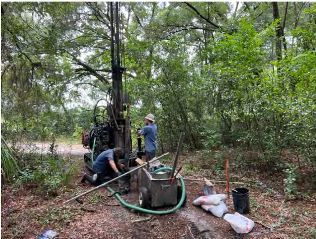
Photograph No. 4: View of soil boring operations at subject property.
