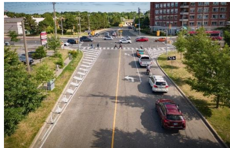
Reduced curb radii speed management.
